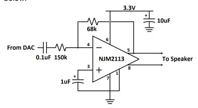
Build your circuit and connect it to a 3.3V power source. Use a function generator to input a 2.4V peak-to-peak sinusoid of about 1kHz and verify the outputs of the NJM2113 (pins 5 and 8) show a sinusoid of at least 1V peak-to-peak. If not, check your circuit or consult the NJM data sheet for more information.
