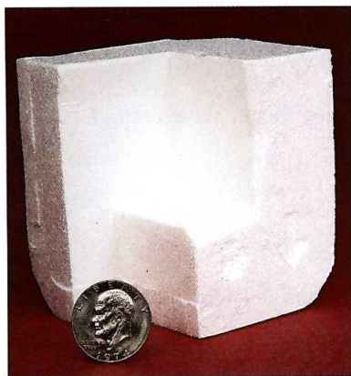
Figure 2.8 Both of these items have a mass of 23 grams, but very different volumes. The volume differences result from the two items having different densities.
