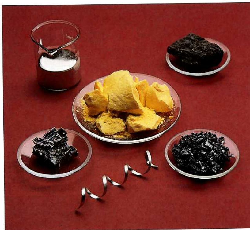
Figure 1.10 Outward physical appearance of selected naturally occurring elements. Center: Sulfur. From upper right, clockwise: Arsenic, iodine, magnesium, bismuth, and mercury.
